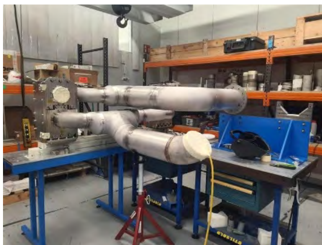
Cooling pipework being welded outside the CAL
